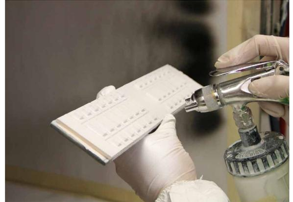
Once the part receives its coating, proper handling is required to prevent issues with the finish. Improper handling will result in contaminants falling on the wet paint, damaging the finish and increasing the likelihood of adhesion problems. In many commercial settings, parts move through a paint booth on a hanging conveyor thereby avoiding manual handling of the wet parts until after curing in the ovens.
