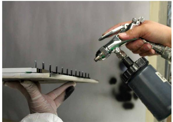
There are several choices to ensure good paint adhesion when it comes to pre-finishing metal parts such as aluminum. Two popular and effective choices are chem film and anodizing. Chem film, also known as chemical conversion coating, is a process that applies a chromate conversion coating primarily on aluminum and aluminum-related alloys. This process promotes good paint adhesion while conducting an electrical charge and provides some protection from corrosion.
